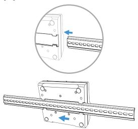
2. Using the appropriate hardware listed above, secure the DIN rail to the charge rack.
