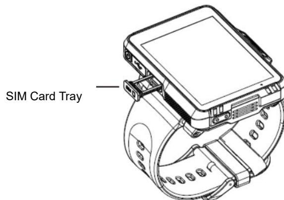
Step 1: Power off the terminal, then pull out the SIM card tray;
