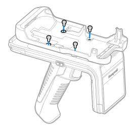
**Note:** The attachment screws ship with the bracket for the mobile computer. The screws are size M3x.5x6. Using a different size screw than those provided with the bracket may damage the RFID reader.
