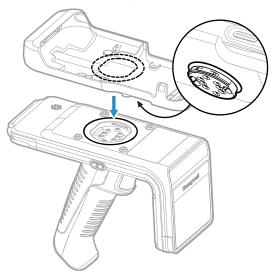
2. Insert the four screws provided with the bracket and tighten.
