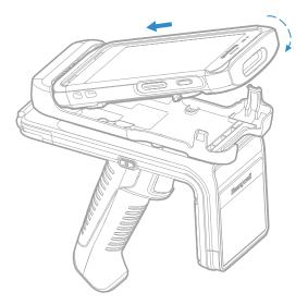
**Note:** When installing the bracket, pay attention to the angle and pressure to avoid damaging the product.
