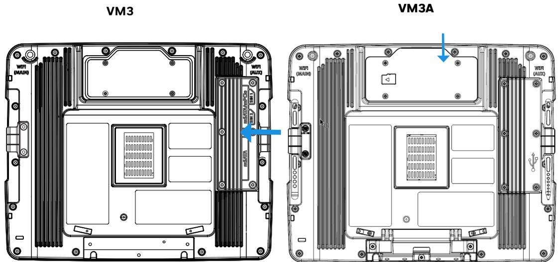
5. Remove the access panel from the opening and press the UPS Battery disconnect button.
