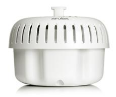
In outdoor and environmentally challenging locations such as oil rigs, mining facilities, and industrial plants, networks need to be protected from extreme temperatures, flammable gases or vapors, and dust concentrations. With Class 1 Division 2 and ATEX Zone 2 certifications, HPE Aruba Networking 570EX Series Access Points deliver reliable Wi-Fi 6 performance to the most extreme environments.
