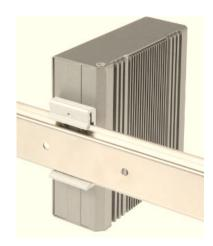
Fasten the DIN-rail bracket by screws **(M3 x 6L)** on the KUBER-1000, suitable for 35mm (W), 7.5mm(H) DIN-rail (Type  $\Omega$ ).
