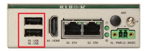
KUBER-1000 provides two USB Type-A 2.0 to connect external device such as mouse, keyboard or external storage device.
