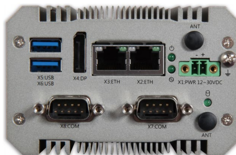
Expanded interface with 1 x RS-232, 1 x RS-232/422/485 (BIOS Configurable)
