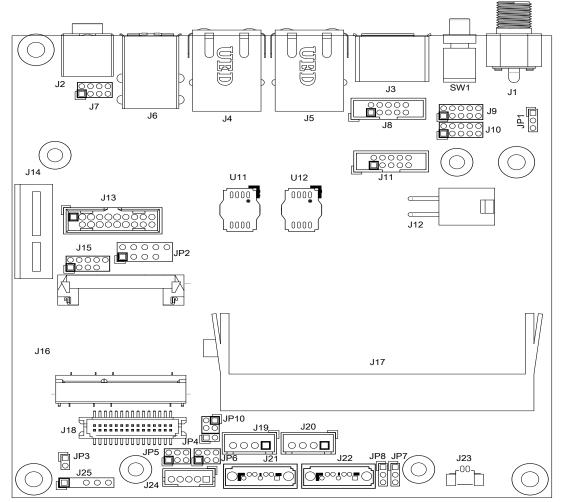
Figure 2-1 NANO-6060 Jumper and Connector Locations
