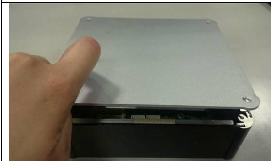
Step 8. Tighten the 4 screws of the back cover
