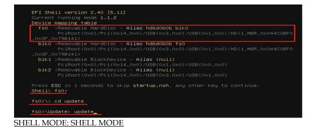
6. When you see the "FPT Operation Passed" message, which means the BIOS update processes finished. Please cut the AC power off and **wait for 10 seconds** before powering on.
