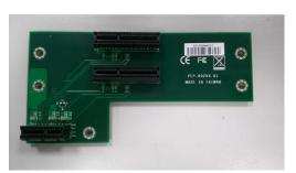
• 1x PCIe x 8 slot (with PCIe x8 signal) & 2x PCIe x 4 slots (with PCIe x4 signal)
