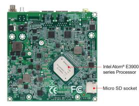
NANO-6062 build with Intel Atom® processor E3900 series. Not only does it operates with TDP under 12W for fan-less applications, but it also supports industrial temperature range from -40°C to 85°C and wide voltage of power input from 12V to 24V. Support four USB 3.0 ports ensures fast data transmission with low-power consump-Gb/s (one of them available as mSATA and
