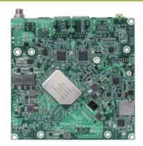
NANO-6063 is based on Intel® Atom® Elkhart Lake family processor. This processor not only supports the range of industrial temperature standard which is from -40°C to 85°C but operates in certain 12W with low-power consumption.
