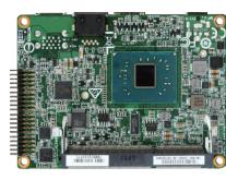
Portwell's PICO-6260 is a palm-sized fan-less PICO-ITX motherboard built with the 14nm Intel® Celeron® processor N3350 (codenamed Apollo Lake SoC).
