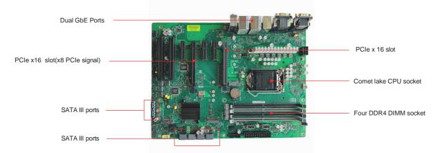
RUBY -D812 is based on Intel® Q470E chipset and Desktop processors including Intel® 10 th Gen Core™ i3/i5/i7 SKU. This board supports DDR4 ,PCIe 4.0, and SATAIII. Those features help you to build high performance and stabile system.
