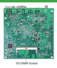
WADE-8079 is based on Intel® Atom® processor E3800 product family with memory and PCI Express controller integrated to support two-channel DDR3L memory and PCI Express 2.0 lanes. Portwell has taken advantage of such technology to furnish a series of products that meets multiple industrial requirements for cost effectiveness, reliable performance and a high level of data integrity and uptime.
