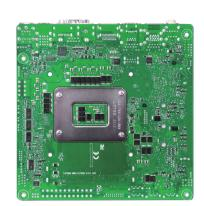
WADE-8213-Q670E is based on Intel® Q670E chipset and 12<sup>th</sup> Gen Intel<sup>®</sup> Core™ i9/i7/i5/i3 desktop processors. It supports multiple display outputs, options of legacy features for industrial applications, GPIO ports, dual LAN as well as rich expandability with PCIe Gen5, M.2 M and M.2 E keys. Featuring rich I/O capabilities and advanced connectivity on a smaller and thinner space-saving platform, the Portwell WADE-8213-Q670E is ideal for a wide range of embedded applications.
