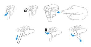
Lift up on the Strap Buckle to unlock the strap. Insert your finger through the Trigger Ring. Pull the excess strap down. Press down on the Strap Buckle. Pull the excess strap through the Strap Loop.
