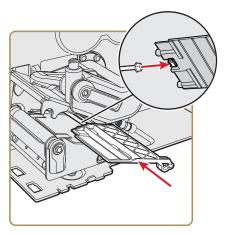
11 Insert the upper media guide all of the way back into the printer. Make sure the plastic pins on the end of the upper media guide fit into the holes in the printer frame and that the end of the upper media guide fits securely over the end of the media post.
