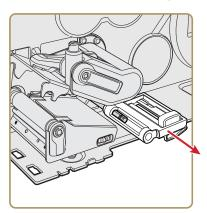
**7** Insert the media path bracket into the printer and attach it to the frame with the Phillips screw.
