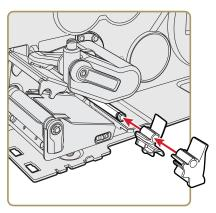
**9** Slide the airline media guide retainer onto the media guide post and secure it in place with the thumbscrew. Make sure it fits securely against the airline media guide closest to the outside of the printer.
