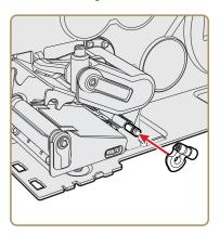
**10** Partially insert the upper media guide into the printer and reconnect the gap sensor cable to the end of the upper media guide.
