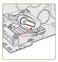
**3** Use a small slotted screwdriver to gently pry the upper media guide loose from the media post. Gently pull the upper media guide away from the printer until you can easily reach the label gap sensor cable.
