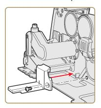
**8** Slide the airline media guides onto the media guide post with the flat side of each guide facing away from the media path.
