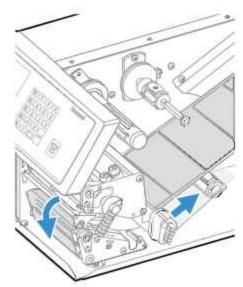
Secure the liner to the take-up hub with the red clip and rotate the hub until the media is pulled tight.
