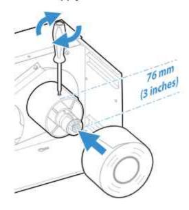
Fit a new roll of media onto the media supply hub and push the roll in as far as it will go.
