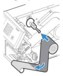
Without releasing the ribbon, turn the printhead lift lever clockwise to lower the printhead and lock the ribbon.
