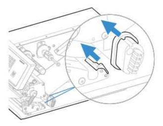
Close the front door and media cover. Make sure that the media runs through the slot in the front door.
