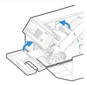
Press the Print/Feed button to advance the media and adjust the media feed.
