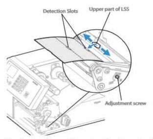
Look at the print mechanism from the front with the printhead lifted to make sure that the point of detection on the upper sensor is aligned with the center of the slots or marks in the media.
