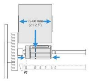
If your ribbon is 88 to 90 mm (3.5 in) wide, compress the ribbon supply bobbin and move it so it snaps into the second groove.
