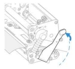
Adjust the position of the red edge guides so that the media is guided with a minimum of play.
