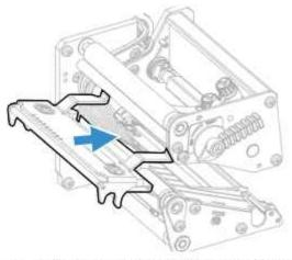
Turn the printhead lift lever clockwise so the magnet engages the printhead bracket.
