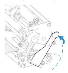
Adjust the position of the red edge guides so that the media is guided with a minimum of play.
