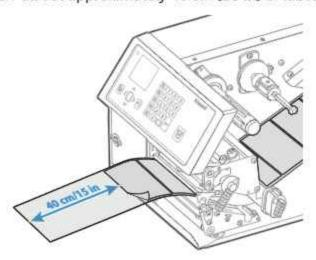
Route the labels around the guide plate and back under the print unit to the take-up hub.
