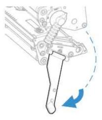
4. Turn the printhead lift lever counterclockwise to raise the printhead.
