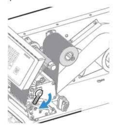
Press the cardboard core at the front end of the ribbon onto the rewind hub. During printing, the rewind hub rotates counter-clockwise.
