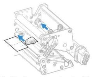
When the pressure arm is centered, tighten the knob to secure the arm. Do not over-tighten the knob.
