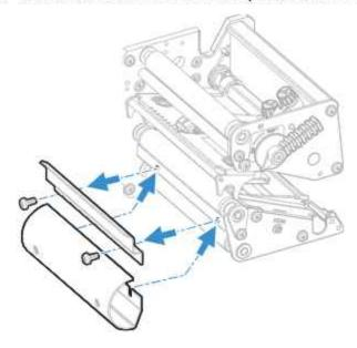
If you are using a media roll with a 76 mm (3 in) core, fit an adapter on the media supply hub.
