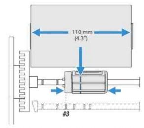
Press the ribbon roll onto the ribbon supply bobbin and route the ribbon through the print unit. Pull out 20 cm (8 in) of ribbon.
