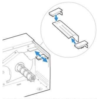
Feed the media through the slot in the rear plate.
