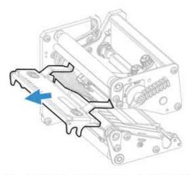
Disconnect the cables from the printhead. Note the snap-lock on the inner connector. Pull at the connectors, not at the cables.
