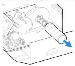
If your are using a media roll with a 76 mm (3 in) core, fit an adapter on the media supply hub.
