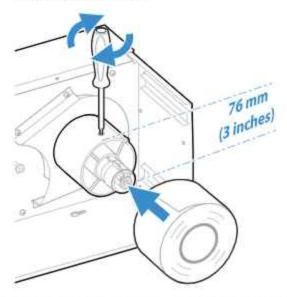
8. Fit a new roll of media onto the media supply hub and push the roll in as far as it will go.
