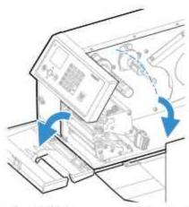
Pull the upper guide straight out and press the snap-lock, lift the edge of the lower guide, and pull the lower guide straight out.
