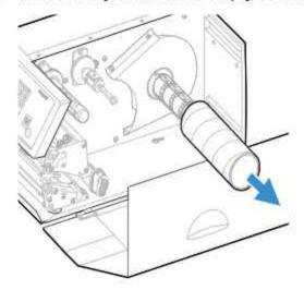
6. If you are using a media roll with a 76 mm (3 in) core, install a 3-inch adapter on the media supply hub.
