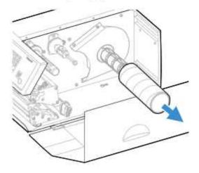
7. If your are using a media roll with a 76 mm (3 in) core, fit an adapter on the media supply hub.
