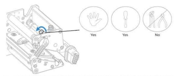
Move the pressure arm inward or outward until the arrow on the tip of the arm is centered with the media.
