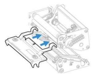
Connect the hooks of the printhead bracket to the headlift shaft. Make sure that the cables are not in the way.
