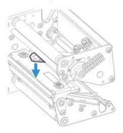
Disconnect the hooks of the printhead bracket from the shaft and pull out the printhead as far as the cables allow.
