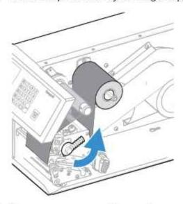
5. If necessary, remove the empty core from the media supply roll post.
