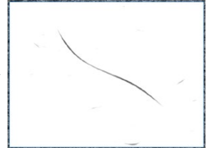
Only linear defects are extracted by ignoring background noise.
