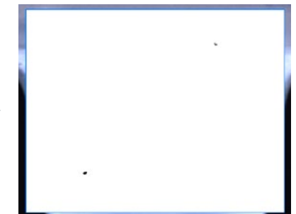
Only defects are extracted by cancelling random shading in real time.
