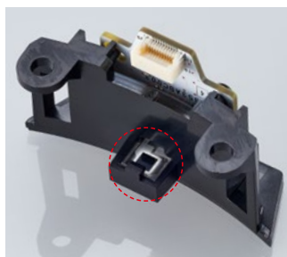
Photodiode and correction circuit within the lighting
