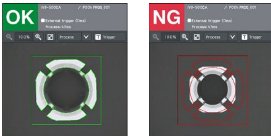
(Appearance-based difference check of metal components)
