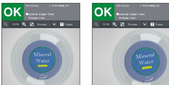
(Mark presence detection with rotational correction)
