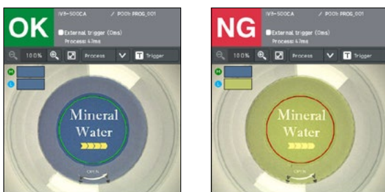
(Colour-based cap difference check)
