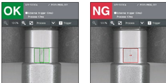
(Type-based difference check of metal components)
