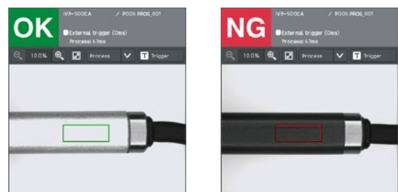
(Type-based difference check of metal components)
