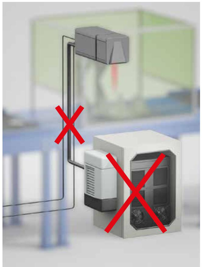
Conventional Fiber Marking System may need additional protective housing for remote controller and complex installation due the limitation of the fiber delivery.
